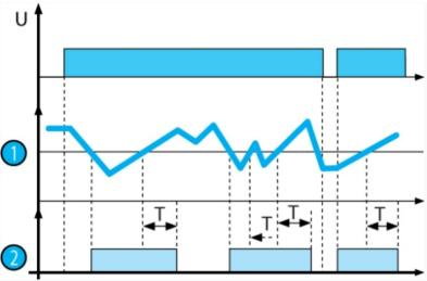
(level : 1 - off delay, function Up LS (Low Sensitivity : 250  $\Omega$  to 5 k $\Omega$ ) or Up St (Standard Sensitivity : 5 k $\Omega$  to 100 k $\Omega$ ) or Up HS (High Sensitivity : 50 k $\Omega$  to 1 M $\Omega$ ).
