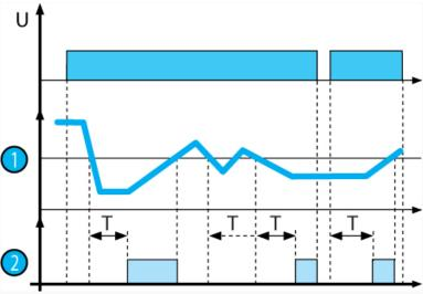
$(level: 1 - on \ delay, \ function \ Up \ LS \ (Low \ Sensitivity: 250 \ \Omega \ to \ 5 \ k\Omega), \ Up \ St \ (Standard \ Sensitivity: 5 \ k\Omega \ to \ 100 \ k\Omega), \ Up \ HS \ (High \ Sensitivity: 50 \ k\Omega \ to \ 1 \ M\Omega).$
