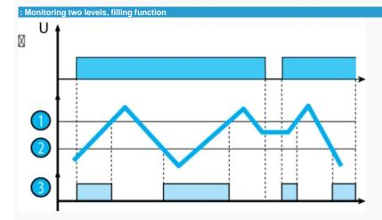
(level : 2, function Up LS (Low Sensitivity :  $250~\Omega$  to  $5~k\Omega$ ) or Up St (Standard Sensitivity :  $5~k\Omega$  to  $100~k\Omega$ ) or Up HS (High Sensitivity :  $50~k\Omega$  to  $1~M\Omega$ ).
