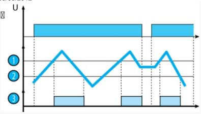
(level : 2, function Dwn LS (Low Sensitivity : 250  $\Omega$  to 5 k $\Omega$ ), Dwn St (Standard Sensitivity : 5 k $\Omega$  to 100 k $\Omega$ ), Dwn HS (High Sensitivity : 50 k $\Omega$  to 1 M $\Omega$ ).
