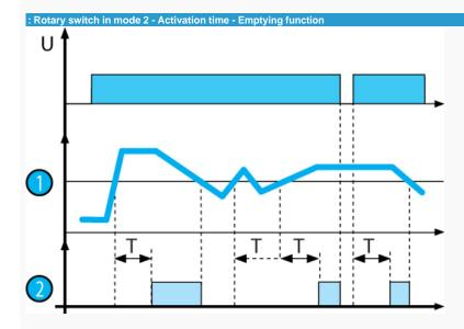
$(level: 1 - on \ delay, \ function \ Dwn \ LS \ (Low \ Sensitivity: 250 \ \Omega \ to \ 5 \ k\Omega), \ Dwn \ St \ (Standard \ Sensitivity: 5 \ k\Omega \ to \ 100 \ k\Omega), \ Dwn \ HS \ (High \ Sensitivity: 50 \ k\Omega \ to \ 1 \ M\Omega).$
