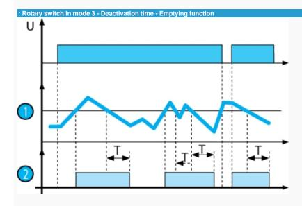
$(level: 1 - off \ delay, \ function \ Dwn \ LS \ (Low \ Sensitivity: 250 \ \Omega \ to \ 5 \ k\Omega) \ or \ Dwn \ St \ (Standard \ Sensitivity: 5 \ k\Omega \ to \ 100 \ k\Omega) \ or \ Dwn \ HS \ (High \ Sensitivity: 50 \ k\Omega \ to \ 1 \ M\Omega).$
