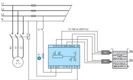
1 A fast-blow fuse or cut-out
